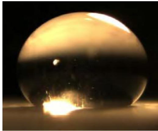
Figure 2. Image of contact angle experiment of SC-15 Part A. Image courtesy of reference 25.
