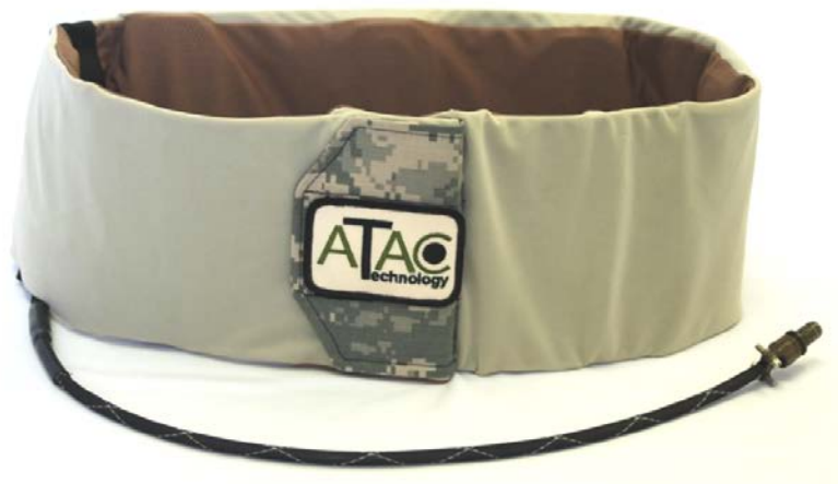
Fig. 5 Prototype dual-row belt. Each belt contained a row of 8 C-3 factors and a row of 8 EMR factors.
