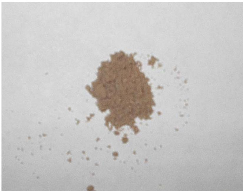
Figure 1. Cryogenically ground polymer powder.
