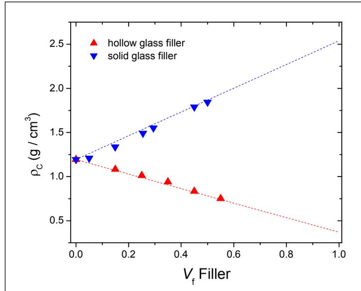
Figure 5. Plots of composite density vs. volume fraction of filler for composites filled with hollow glass spheres ( $\blacktriangle$ ) and solid glass spheres ( $\blacktriangledown$ ). The ROM (equation 1) is used to predict the experimental densities. Density measurements were precise to  $\pm 0.02 \text{ g/cm}^3$ .
