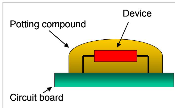
Figure 1. A schematic of an encapsulating potting compound showing the coverage of a surface mounted device.
