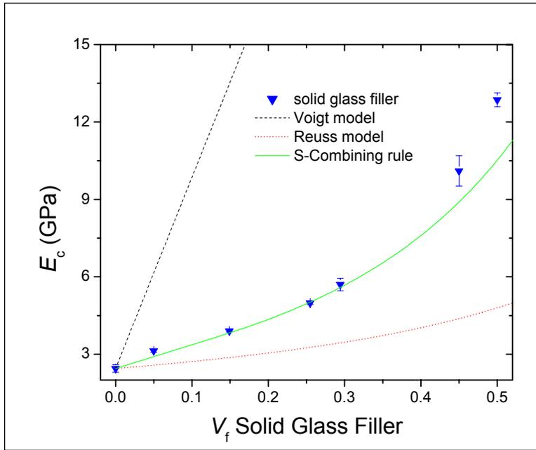
Figure 8. Plot of experimental composite modulus vs. volume fraction of solid glass filler along with theoretical predictions via the S-Combining Rule, Voigt model, and Reuss model.
