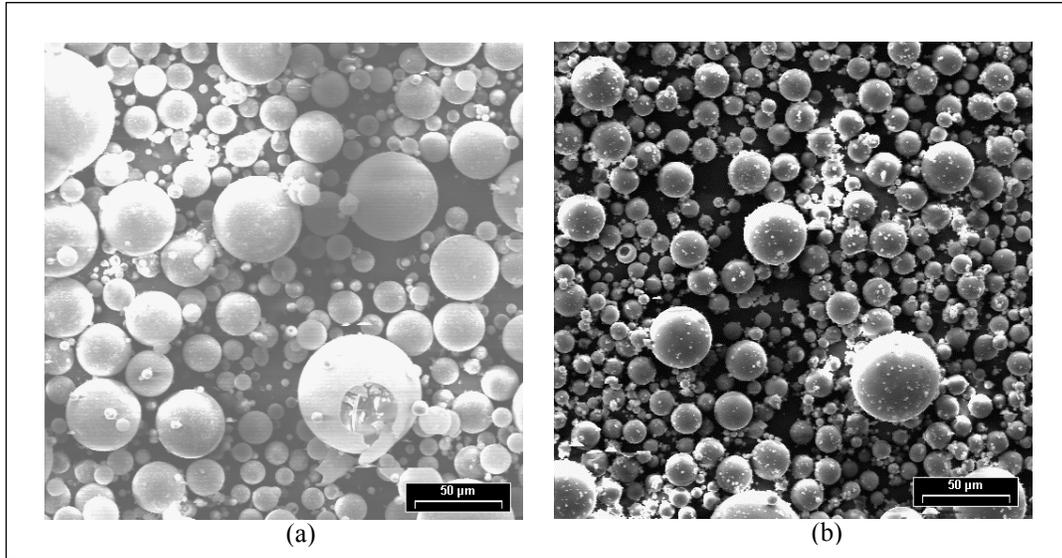
Figure 4. SEM images of the (a) hollow and (b) solid glass fillers.
