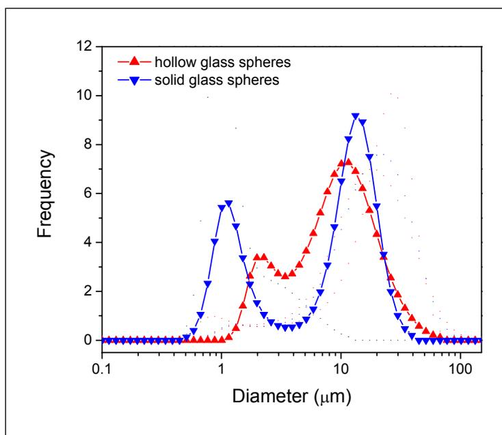
Figure 3. Particle size distributions for the hollow ( $\blacktriangle$ ) and solid ( $\blacktriangledown$ ) glass fillers.
