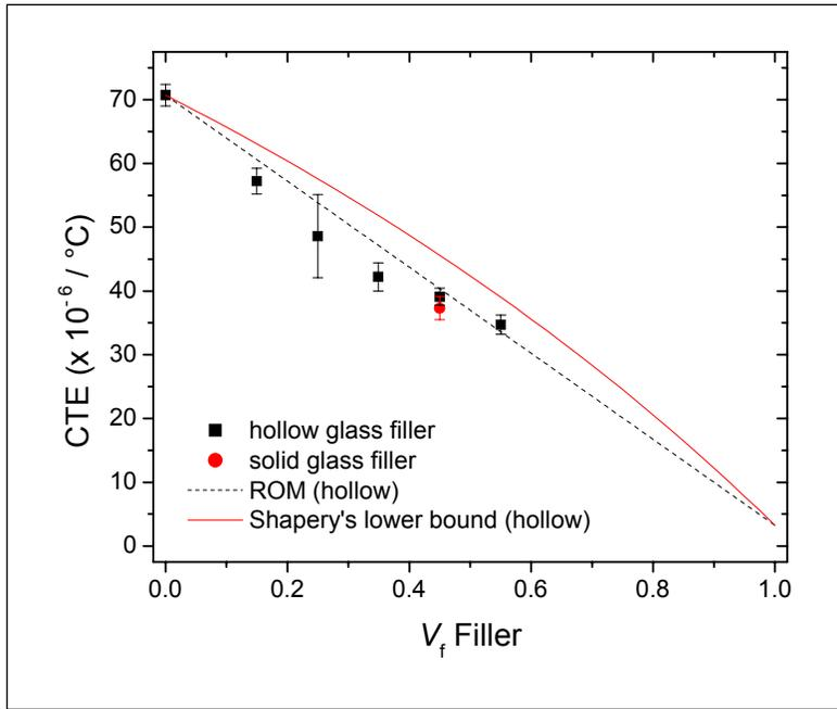
Figure 6. Composite CTE vs. volume fraction of hollow glass filler (■). Composite CTE at  $V_f = 0.45$  solid glass filler (●) illustrated for comparative purposes. ROM and Schapery's lower bound fit to hollow glass filled composite data.
