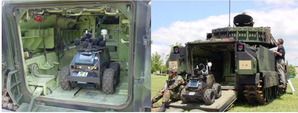
Figure 8. Robotic Scout in Bradley Fighting Vehicle.
