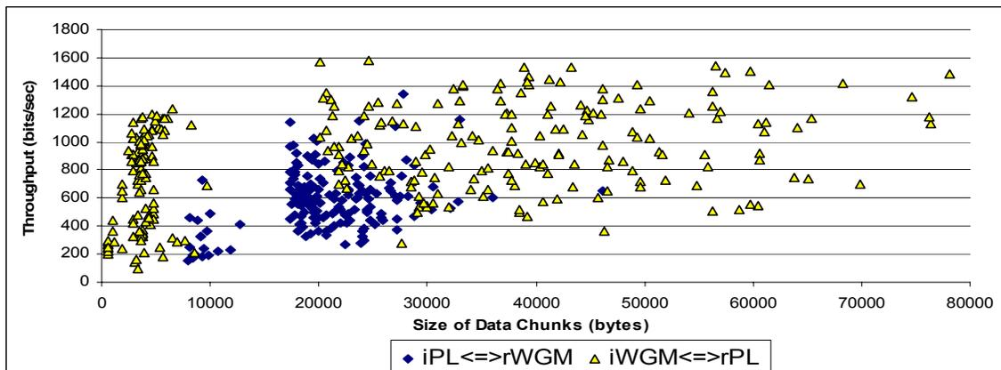
Figure 11. Throughputs versus sizes of data chunks.
