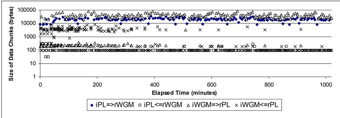
Figure 8. Sizes of data chunks transmitted over the SINGARS link.
