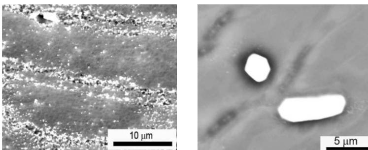
Fig. 1. (a) SE micrograph depicting shear localization and precipitation gradients (b) BSE micrograph showing cuboidal  $\text{Mg}_2\text{YZr}_{0.3}$  and plate shaped  $\text{Mg}_{41}\text{Nd}_5\text{Zr}$  intermetallics
