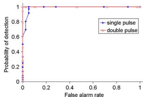
**Fig. 4** ROC curves for the discrimination of RDX and diesel fuel residues on aluminium generated from the first principal-component scores based on atomic emission ratios for both single and double-pulse LIBS [36]. The double-pulse ROC curve represents complete discrimination between the two residues (100% true positives with 0% false positives)
