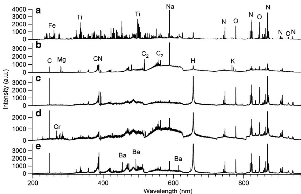
from clutter objects by use of LIBS, different types of mines can be discriminated from each other with a high degree of success.
