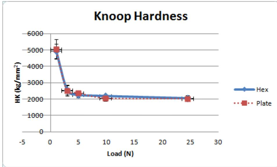
Figure 5. Load-HK curve.
