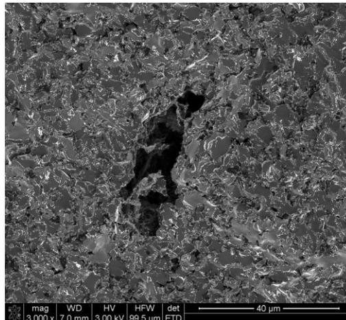
Figure 4. SEM of pore in the weakest sample.
