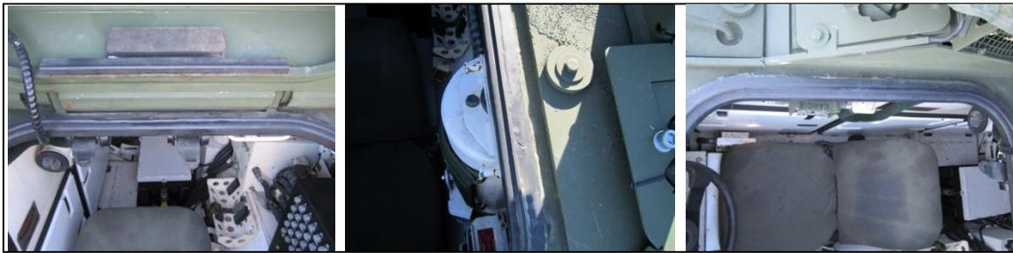
Figure 9. Stryker (ICV-0269-03) access hatch seal at 6-month inspection.
