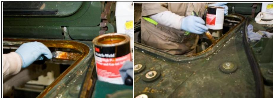
Figure 5. Adhesive application to the steel channel of the Stryker access hatch.
