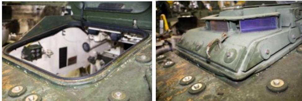
Figure 8. Bonded access hatch seal (left) and hatch door closed (right).
