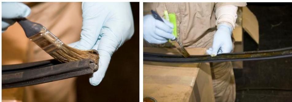
Figure 6. Adhesive application to the rubber seal of the Stryker access hatch.
