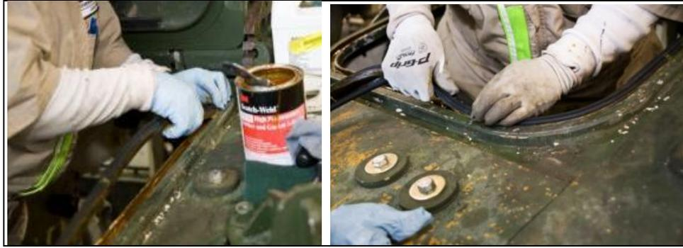
Figure 7. Bonding seal to the steel channel of the Stryker access hatch.
