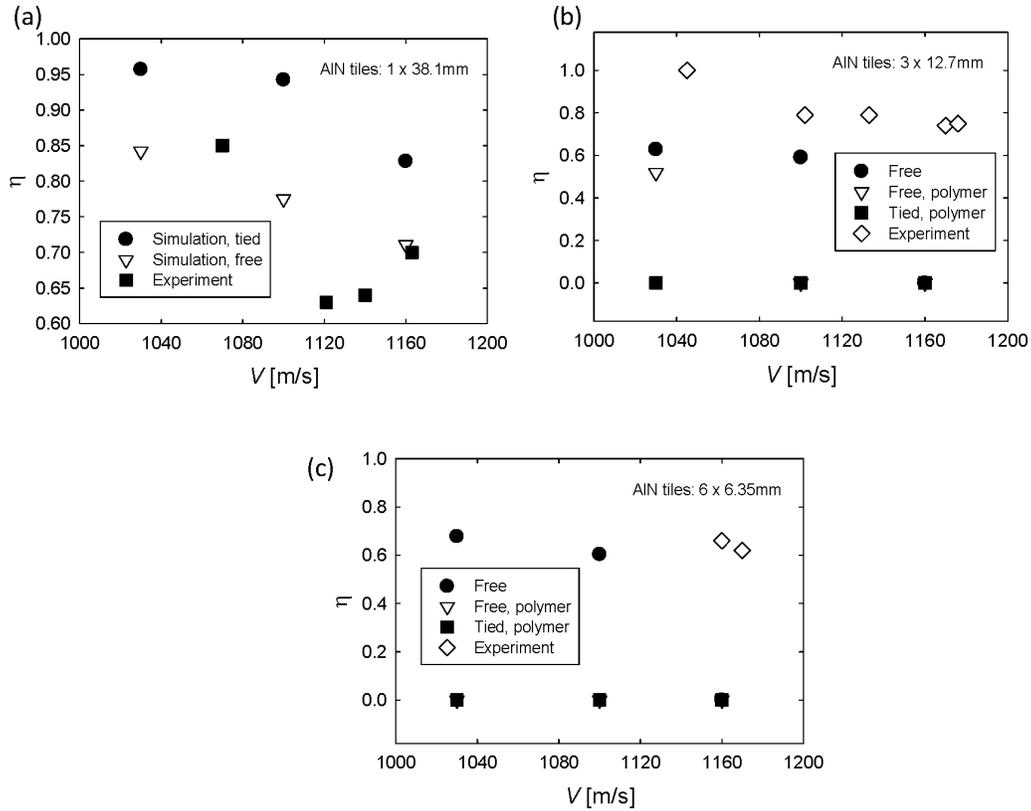
**Fig. 4 Ballistic efficiency vs. impact velocity for ceramic-metal targets from simulations and experiments: a) 1 tile, b) 3 tiles, and c) 6 tiles**
