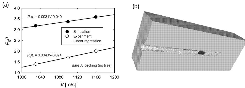
**Fig. 2 Penetration into bare aluminum backing material: a) depth vs. impact velocity for simulation and experiment<sup>1</sup> and b) simulation result at impact velocity of 1,030 m/s**
