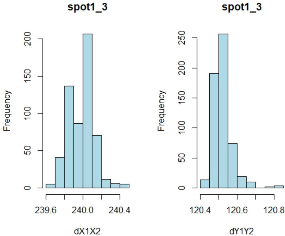
**Fig. 4** Typical scatter of distance measurements in millimeters at spot-1/scan-3 data subset. True value for dX1X2 = 239.08 mm; true value for dY1Y2 = 119.53 mm.
