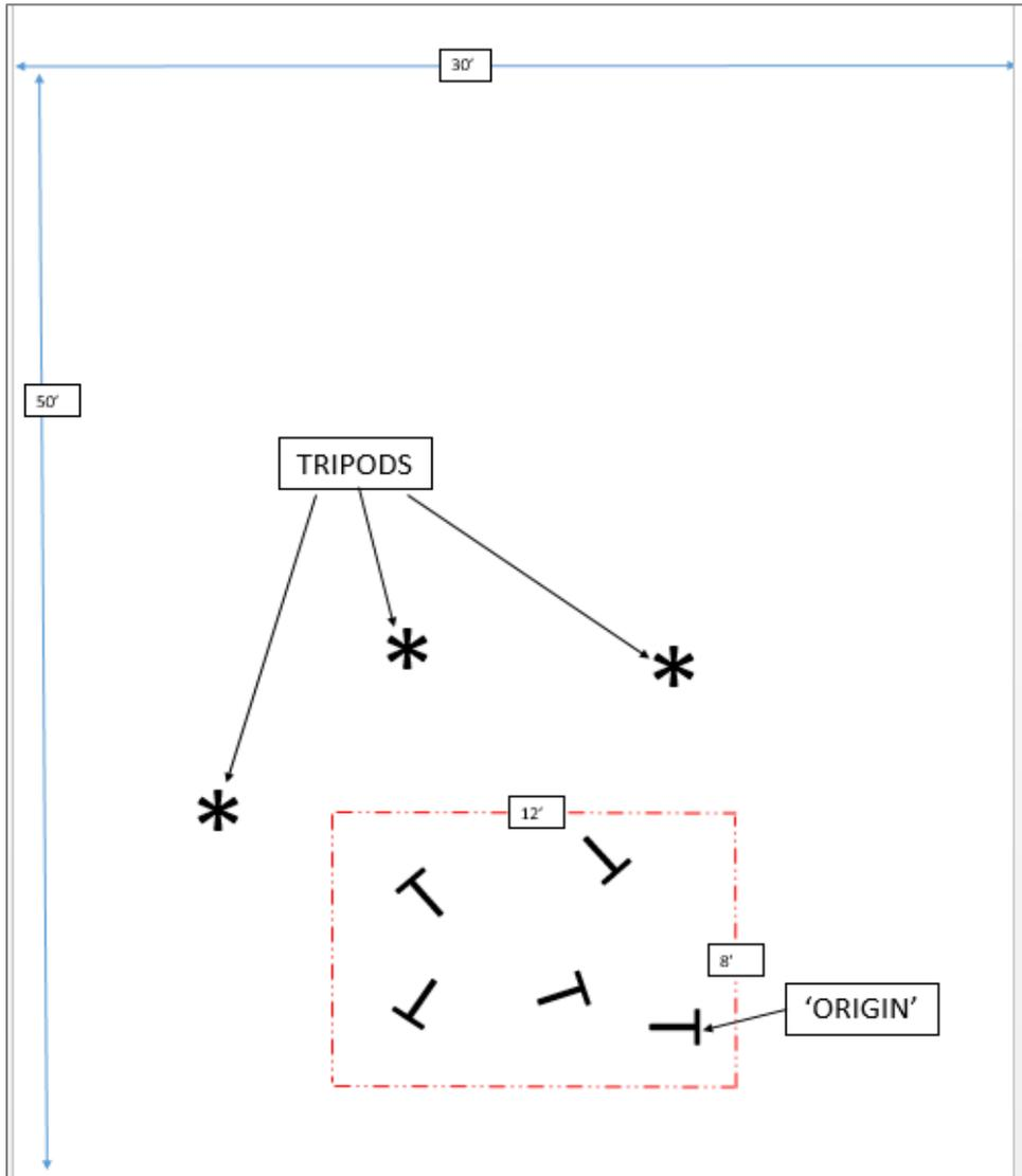
**Fig. 2** Vicon Space (floor) and the Wand locations for the experiment (locations are approximate)
