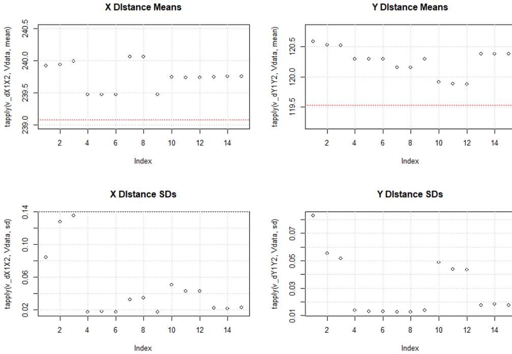
**Fig. 3** Means and standard deviations for X1-X2 and Y1-Y2 distance measures in millimeters. Note that the dotted horizontal lines in the Means plots indicate the true values of 239.08 and 119.53 mm, respectively.
