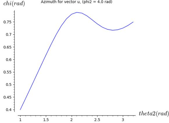
**Fig. 3 Colatitude angle of the second-order invariant vector  $\vec{u}$  as a function of MSR colatitude angle  $\theta_2$  of  $\vec{OP}_2$  ( $\phi_2$  is fixed)**
