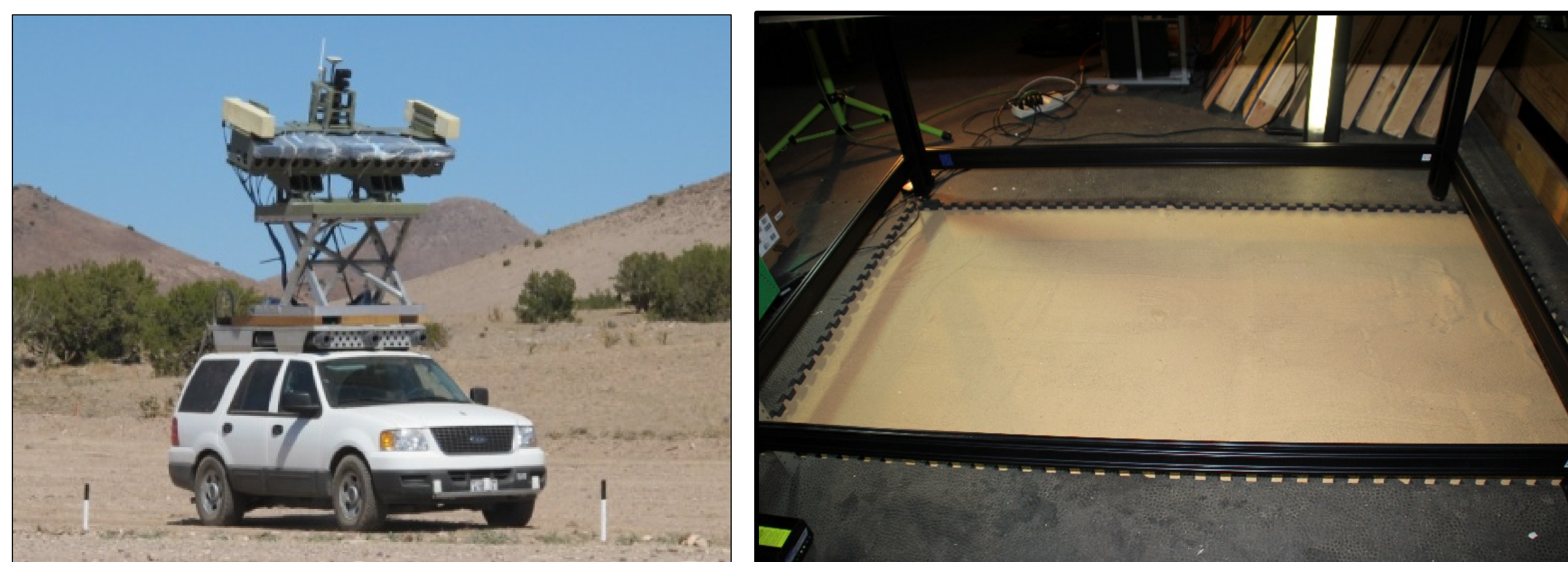
Forward Looking UWB Radar Testbed (left); 2D Scanner Sandbox (right)
