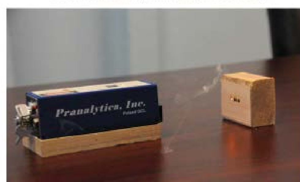
Miniaturization: Battery Operated, 3 W Output Collimated Beam; 5 mm dia (not focused)
