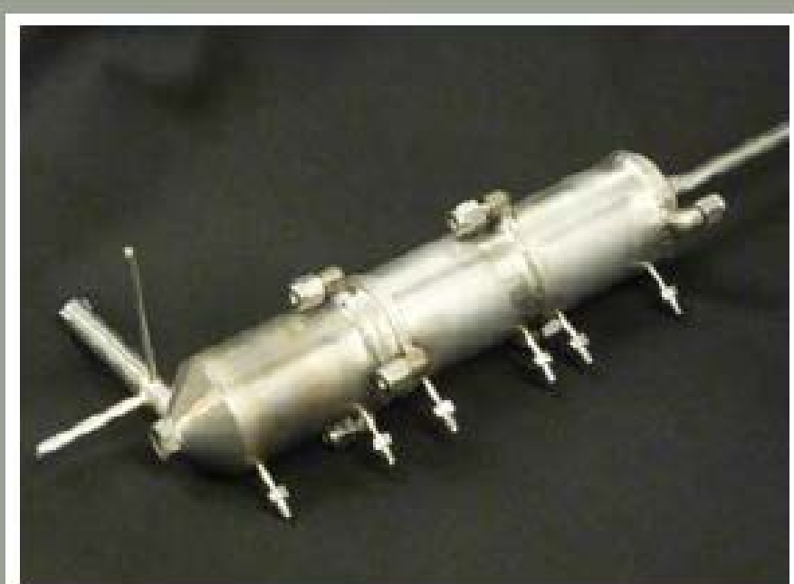
FUEL PROCESSOR: RENEWABLE HYDROGEN FOR PORTABLE POWER
