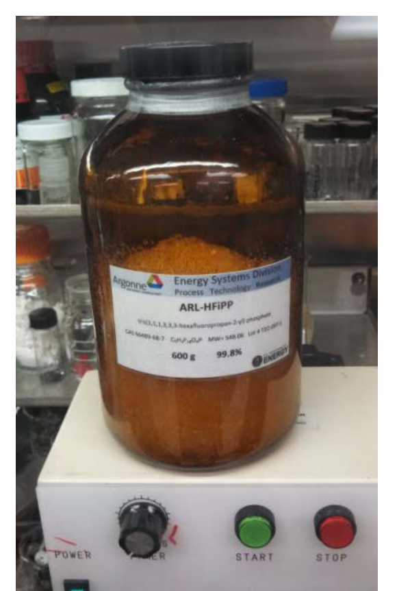
Scale-up of ARL high voltage electrolyte additive
