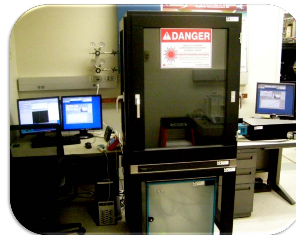
Combined Atomic Force Microscopy and Raman
