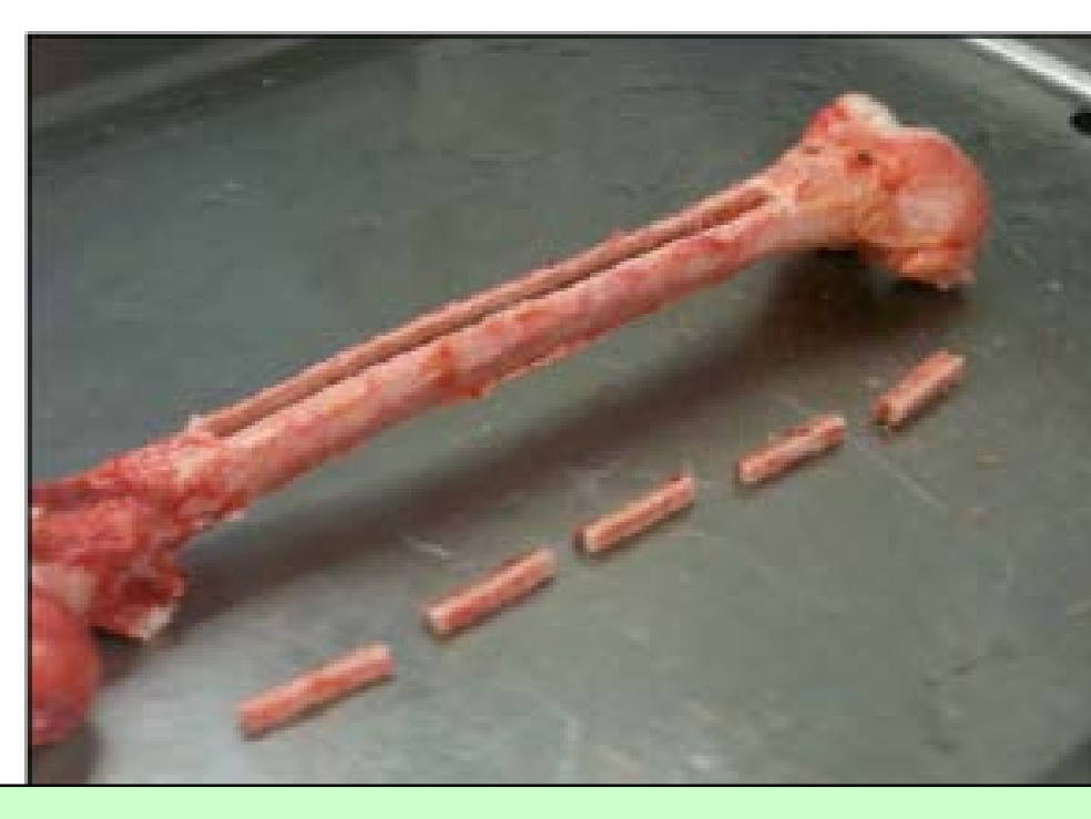
Human femur with extracted rough cut specimens
