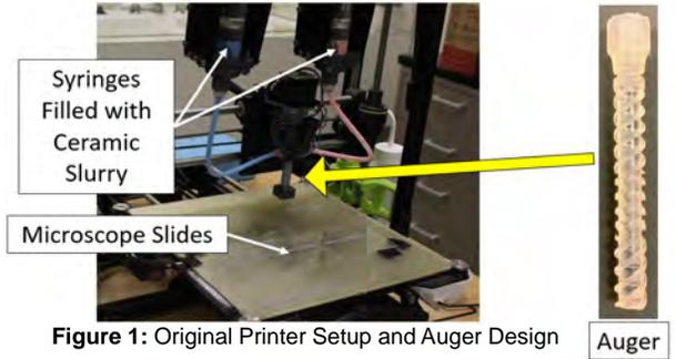
Figure 1: Original Printer Setup and Auger Design
