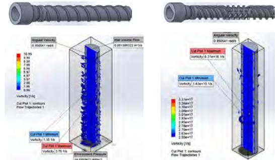
Figure 4: Auger Vorticity Profile
