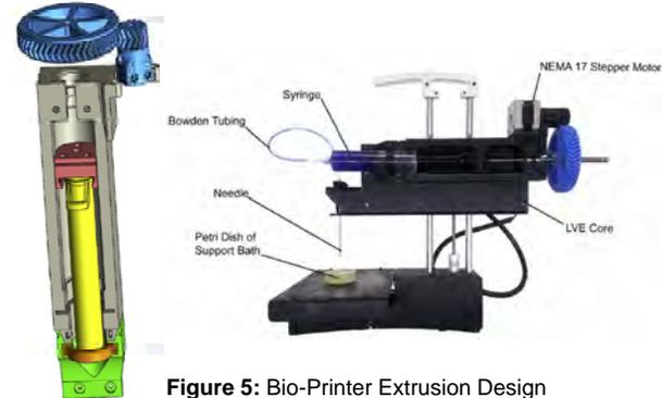
Figure 5: Bio-Printer Extrusion Design
