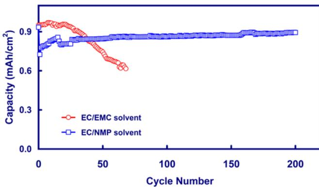
*Use of a lactam-based solvent in electrolyte significantly increases capacity retention of Li-ion batteries (source: SEDD)*
