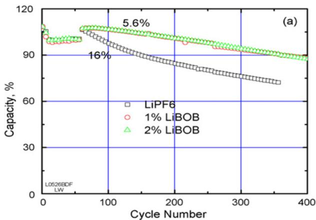
Solvent additive increases capacity retention of Li-ion batteries at 55 °C (Source: J. Power Sources, 163, 2007, 1074-1079)
