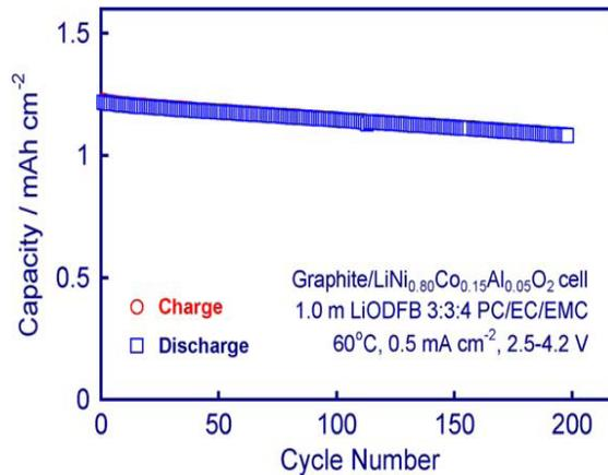
The chart illustrates performance of a LiDOBF-based cell, which suffers only about 10% capacity loss after 200 cycles at 60°C while maintaining nearly 100 percent charge efficiency
