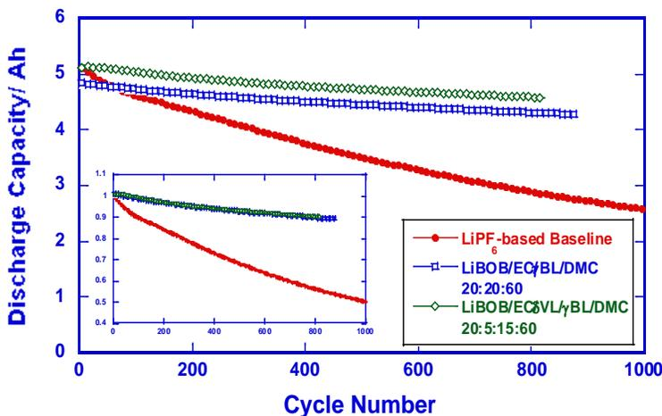
More than 90 percent capacity retention at 800 cycles at  $60^\circ\text{C}$
