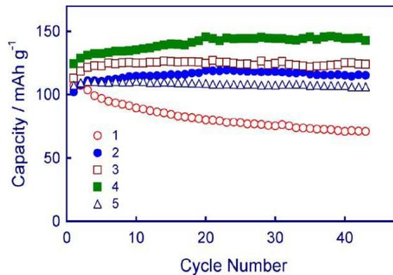
All the cells with  $\text{LiFePO}_4\text{-C}$  cathodes (2-5) exhibited much more stable capacity with increasing cycle number than the  $\text{LiFePO}_4$  control cell. (source: SEDD)
