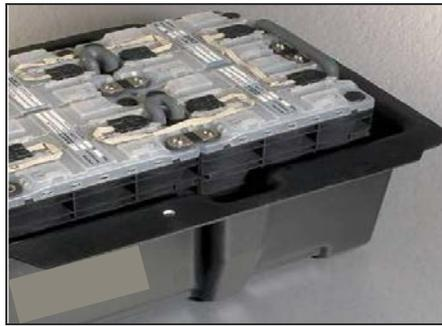
*The SEDD innovation increases cell chemistry kinetics, creating cells that deliver power much more rapidly and make better use of EV regenerative braking (Image sources: DOE)*
