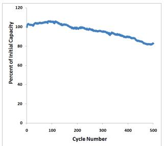
ARL innovation produces capacity retention of more than 80 percent after 500 cycles (source: ARL)
