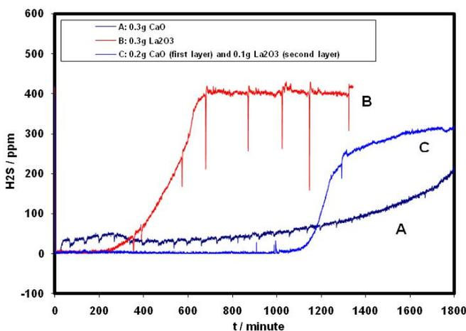
*Desulfurization results comparing two single sorbent systems (A and B) and ARL invention (C). Data illustrate that with 420 ppmv starting concentration, the ARL system maintains low ppmv levels of H<sub>2</sub>S far longer and more consistently than single sorbent systems (Image source: ARL)*
