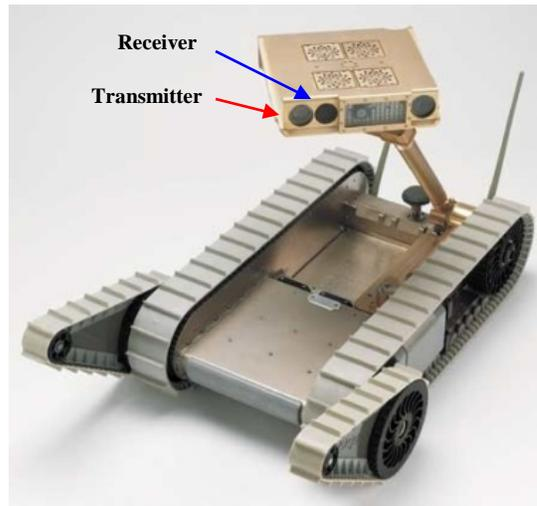
ARL LADAR-based system mounted on iRobot Explorer PackBot (Image source: ARL)
