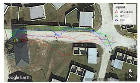
Path difference metrics: learned robot trajectories vs human-driven "ground truth" on "covert" navigation task
