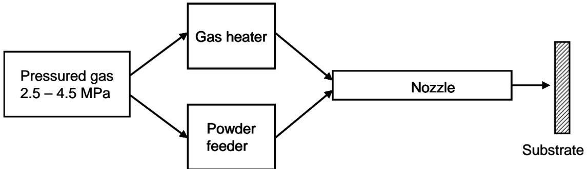
FIGURE 1. High-pressure system.
